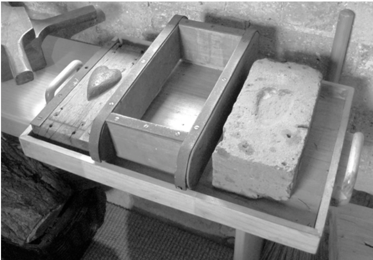
Figure 5. Brickmaking equipment: the stockboard with heart-shaped kick (left), the mould (centre), and a finished brick (right).
